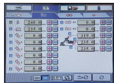
The guide and buckle positions can be fine-tuned by 0.1 mm with a simple touch of the + or - button.
