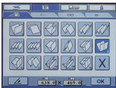
Setup is completed by selecting the desired fold pattern and inputting the sheet size.
