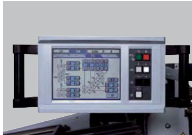
Roller Gap Adjustment Screen The number of sheets to be inserted into each gap adjust lever is indicated for quick setup.
