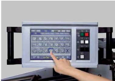
Fold Pattern Setup Screen Setup is completed by selecting the desired fold pattern and inputting the sheet size.
